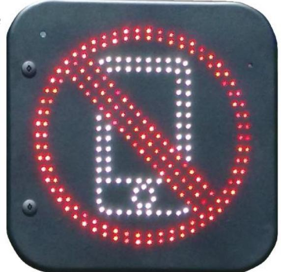
The technology can detect if a driver is using Bluetooth, and will therefore not trigger the warning sign. However, any system finds it hard to differentiate between users in the car, we accept that some activation might be triggered by non-driving occupants. The vast majority of activation's will relate to drivers, and we don't see a problem when passengers activate the sign. In fact, it's all part of the education message that using a phone when driving is not only illegal but very dangerous.
